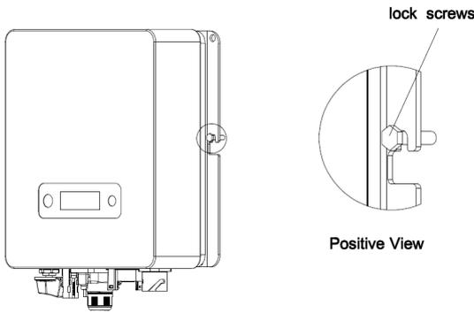
Step 3: Plug Grid side connector into AC connector of inverter end, rotate and tighten clockwise.
