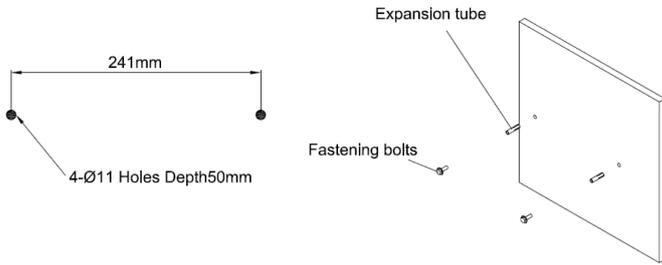
Step 2: Place the inverter on the wall-mounted bracket and install the fix screw.
